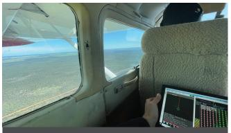
CONDUCTING AERIAL LASER SCANNING (LIDAR) SURVEY
